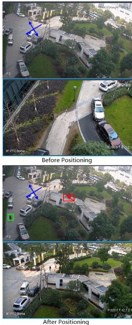
Figure 4-114 3D positioning (Zoom out after positioning)
